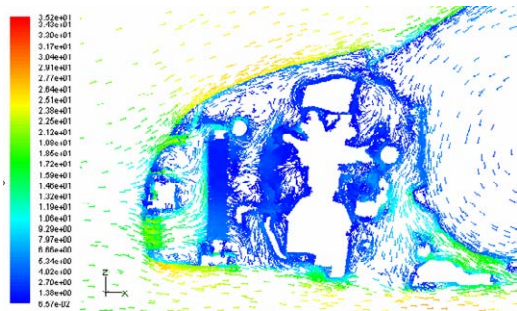
Velocity Vectors Colored By Velocity Magnitude (m/s) Feb 05, 2011 FLUENT 6.3 (3d, pbns, zshw)
